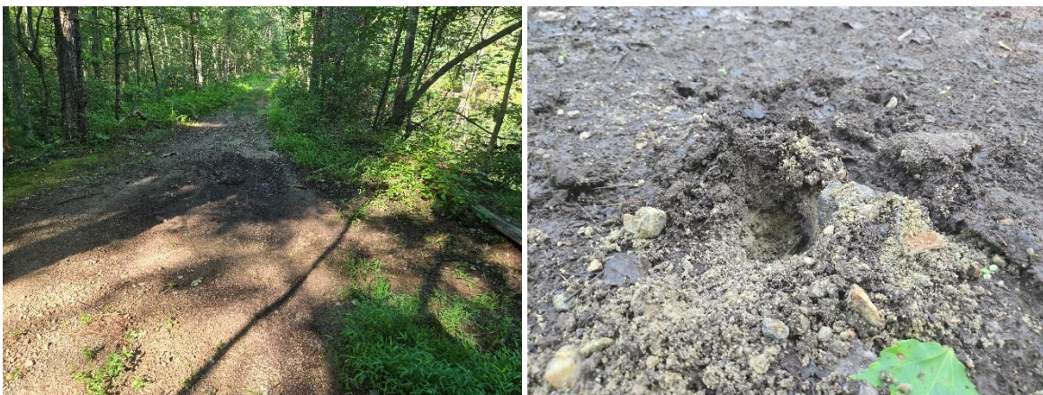
Left Photograph: View of saturated area likely from WF-A Series BVW overtopping Right Photograph: Close up of auger pull within saturated area where shallow resistance (compacted gravel) was encountered within the first few inches
